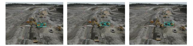
Figure 5. An example of tracking an off-road articulated dump truck (taken over and cropped up: Zhu *et al.*, 2016)
