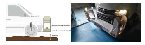
Figure 2. A view of the measurement vehicle Hawkeye 2000
