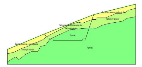
Figure 7. Cross section of soil layers
