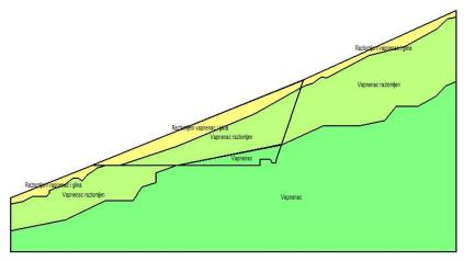
Figure 3. Cross section of soil layers
