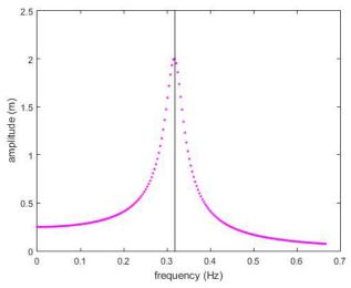
Figure 2. Frequency response of a linear SD system (FRD)
