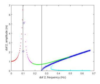
Figure 7. Frequency response of a nonlinear system with two degrees of freedom (stage two)
