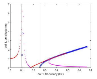
Figure 6. Frequency response of a nonlinear system with two degrees of freedom (stage one)
