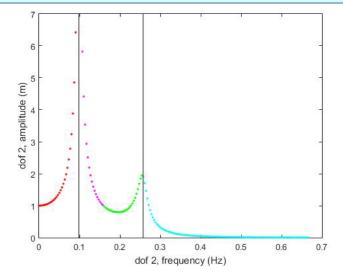
Figure 5. Frequency response of a linear system with two degrees of freedom (stage two)
