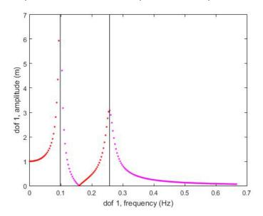
Figure 4. Frequency response of a linear system with two degrees of freedom (stage one)
