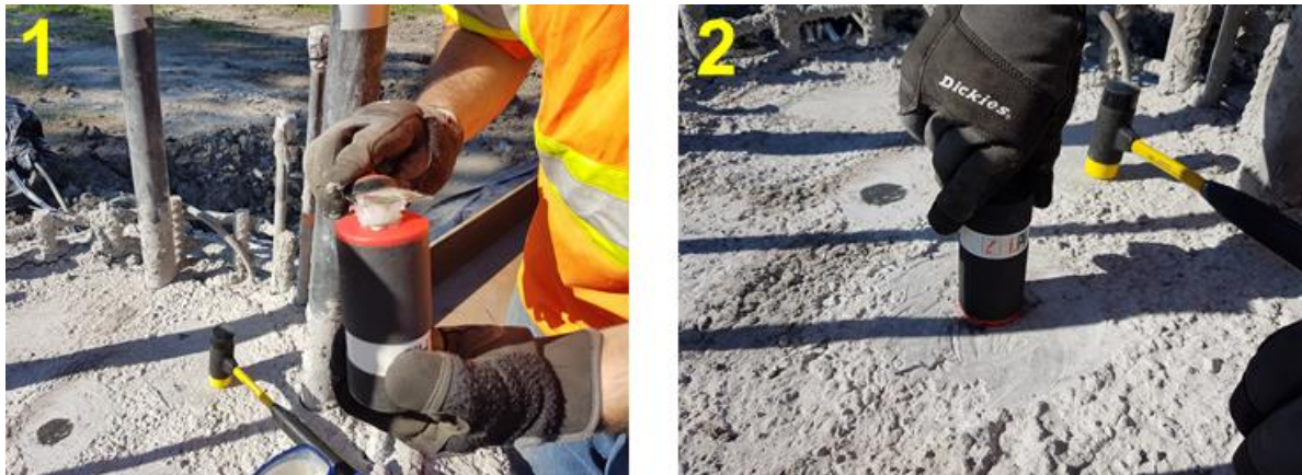
Figure 6. The method of placing the sensor on the pile head [30]
