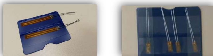
Figure 10. - Strain gauges for concrete (left) and steel (right)
