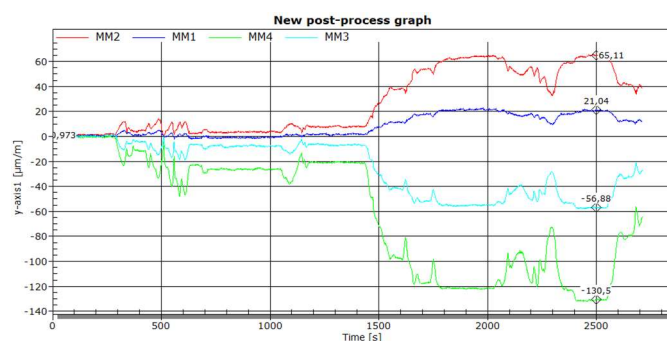
Figure 28. - Time history of strains for the change in flange and slab thickness – right
