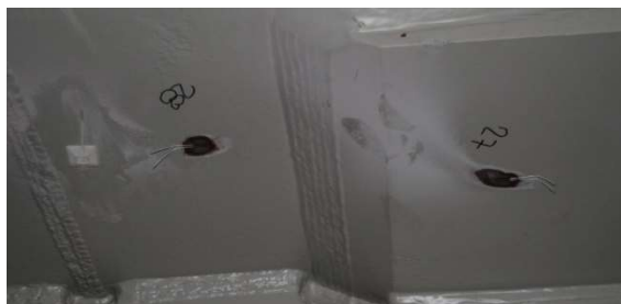
Figure 29. - Strain gauges for measuring strains for the change in flange thickness
