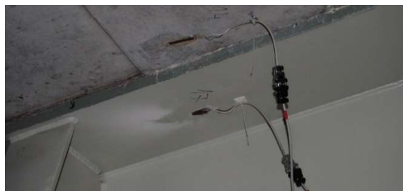
Figure 19. - Strain gauges for measuring strains on concrete and steel structures
