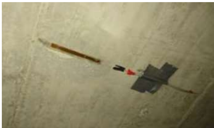
Figure 5. - Strain gauge at the test location
