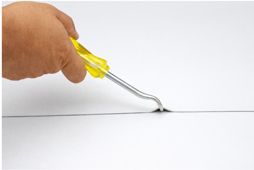
Figure 10. Manual control using a weld tester [1]
