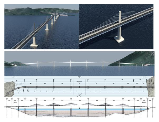
Figure 10. View of the bridge, plan view and longitudinal section
