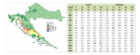
Figures 6, 7. Spatial distribution of basic wind speed and expected 10-minute wind speed, as well as the corresponding probability (P%) for T-year return periods obtained from the measurement data at the meteorological stations of Ploče and Komarnain the period 2005 - 2014
