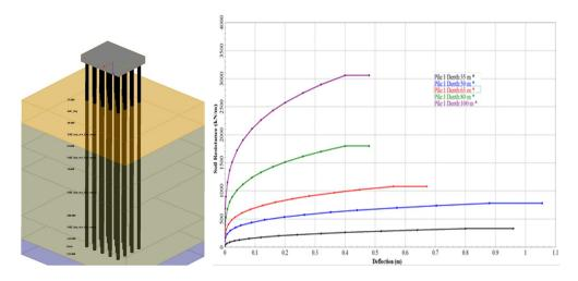
Figure 17. View of "p-y" curves / nonlinear behavior of foundation soil - clay at different depths
