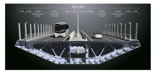
Figure 9. The bridge superstructure with traffic surfaces
