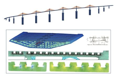
Figure 33. Model of the entire bridge and illustration of fatigue control in superstructure sheet metals
