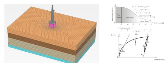
Figure 14. 3D model of the continuum of soil and foundation structure with volume FEM elements
