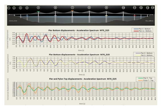
Figure 29. TH analysis results - time dependent displacements of the structure in the transverse direction
