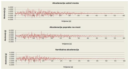
Figure 28. An example of earthquake load - synthetic accelerograms, simultaneously acting longitudinally, transversely and vertically to the bridge (M = 7.5, epicenter distance 100 km)
