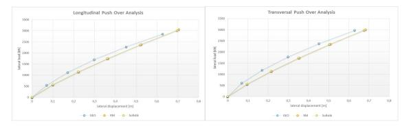
Figures 22, 23. Comparison of results of the "push-over" analysis on the geotechnical model and on the beam model with nonlinear springs
