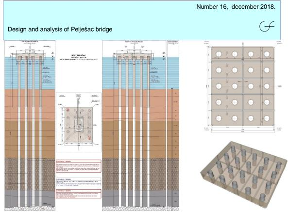
Figure 13. Foundations of piers S7 and S8
