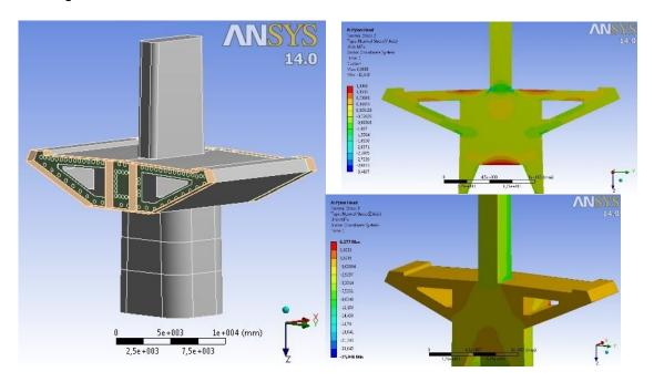
Figure 35. A view of the detailed analysis of the connection of pier, pylon and steel structure with solid elements
