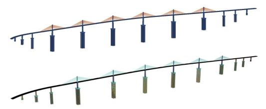
Figure 24. RM Bridge / Bentley model with beam elements and Sofistik model with beam and plate elements
