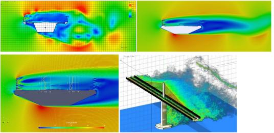
Figure 30. Results of "in-house" CFD analyses of cross section and bridge in the construction stage
