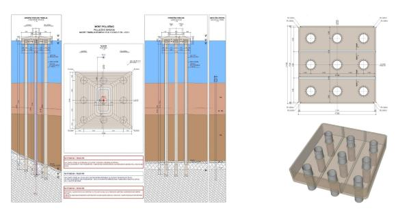
Figure 12. Foundations of piers S3, S4, S11, S12
