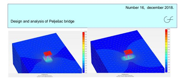
Figure 16. Structural deformations (vertical load + horizontal load 50 MN in the direction of bridge axis and transversely to bridge axis (undrained conditions))
