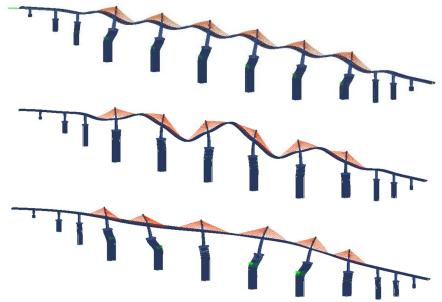
Figure 25. First three oscillation forms of the bridge structure
