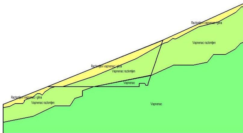
Figure 3. Cross section of soil layers
