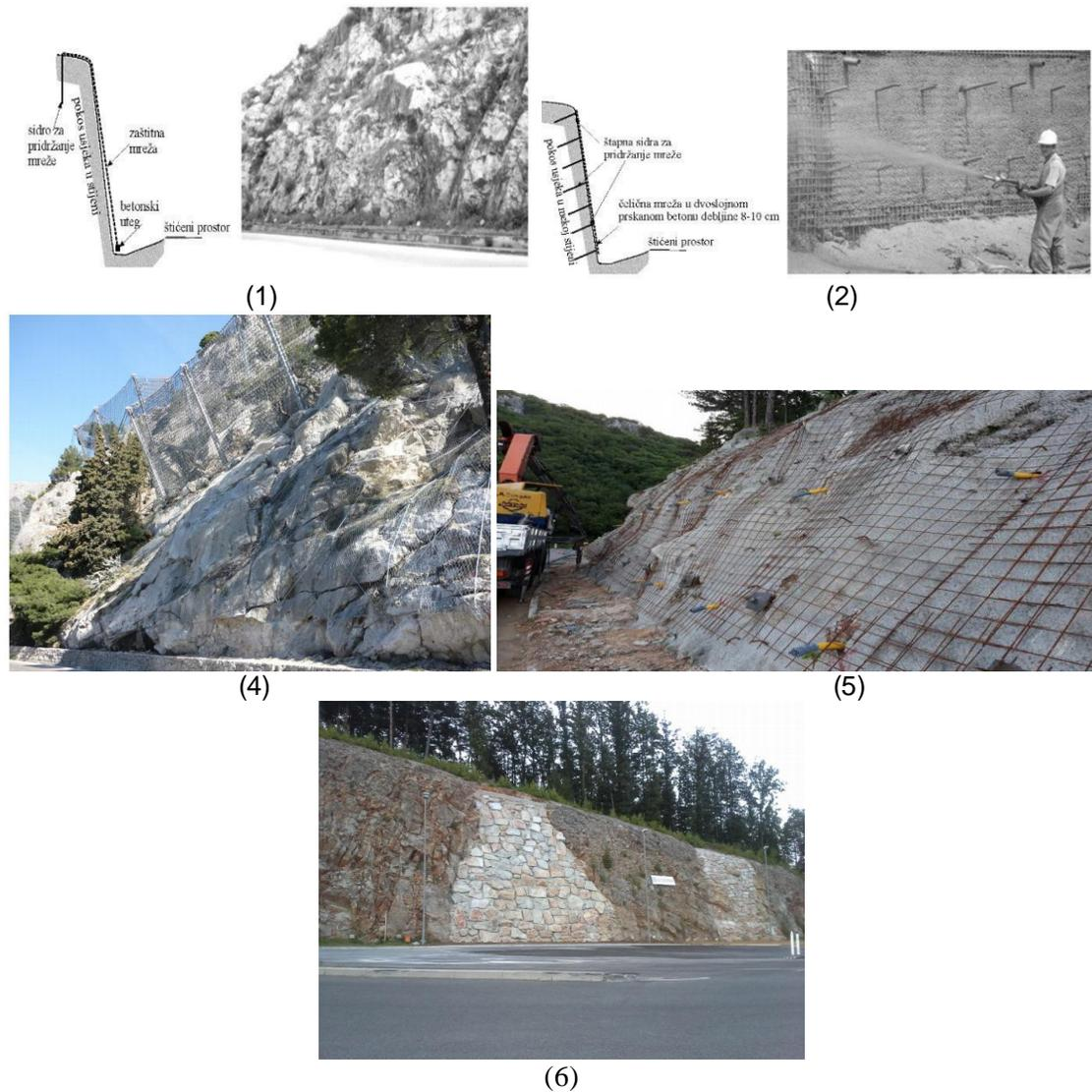
Figure 2. Types of slope protection
