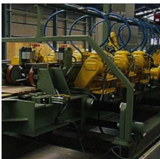
Figure 9. The tile rectification process
