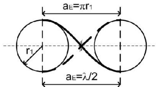
Figure 2. Standing matter wave of a diatomic molecule
