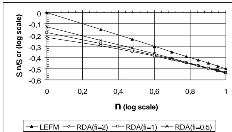
Figure 4. The size effect law of crystal lattice of iron ( $n^* = 2, 1$  and  $0.5$ )
