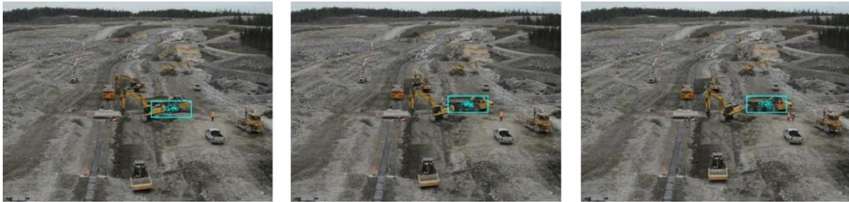
Figure 5. An example of tracking an off-road articulated dump truck (taken over and cropped up: Zhu *et al.*, 2016)
